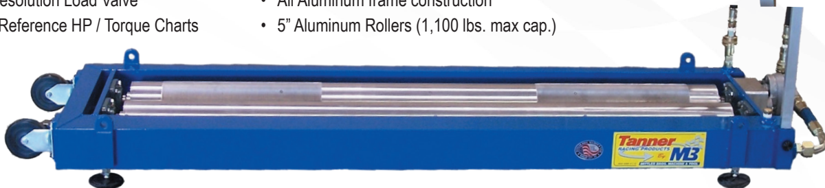
Quarter Midget / Mini Cup / Go-Kart / Bandolero D3 Chassis Dyno 60" Model 99500 $5,750.00
