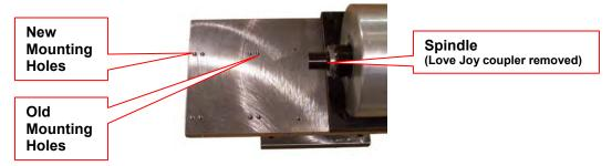
**11.** Slip the two Love Joy coupler halves together with your fingers, being sure the spider is still locked in the "fingers". Tighten the set screws and snug up the motor / gearbox mounting bolts.
