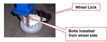
**3.** Turn the stand upright and check caster movement. Be sure the wheel locks work correctly. These casters, when locked, stop the wheel from rolling as well as the locking the swivel.
