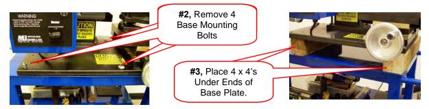
**3.** Raise the machine as shown on *Page 4 Step #5* and place a 4x4 block under each end. Be sure that the 4x4 block on the vise end is even with the edge of the base plate as shown above. Use a C clamp at each end to secure the machine to your work table.
