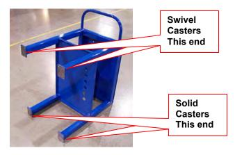
**2.** Using the 5/16" X 1/2" Long Hex Bolts attach the Swivel Casters to the legs on the same end as the handle. Install the bolts from the wheel side and thread into the threaded mounting plate. Attach the solid caster to the opposite legs as shown above. These bolts also thread into the mounting plate from the wheel side. Tighten all bolts.
