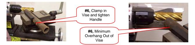
7. If you have the ADJUSTABLE HEIGHT vise, and need to make an OFFSET notch, you need to set the jaw height. This height is set by turning the adjustment screw in or out to get the correct position of the tube in relation to the cutter. The vise must have light pressure on the tube when making adjustments, just snug enough to center the tube in the jaws. Be sure to lock the adjustable jaws once the height is set, using the indicated screws. Once the height is set tighten the vise as usual.
