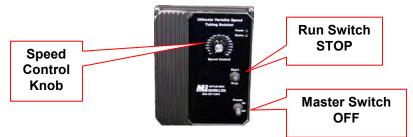
**19.** Turn the **MASTER** switch on and then turn the **RUN** switch on. Turn the speed control knob up and down to cycle the motor. Listen for and clicking or odd sounds. If you hear a clicking sound you will need to loosen the spindle housing bolts and then retighten while the motor is running. This will usually align the Love Joy and quiet the clicking.
