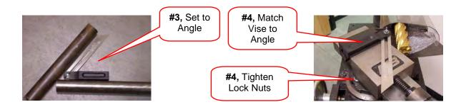
**4.** Set the vise to the correct angle required. Use the supplied <sup>3</sup>/<sub>4</sub>" Combination Wrench to loosen the two vise swivel locknuts. Rotate the vise to the desired angle and lock down by tightening the two lock nuts.
