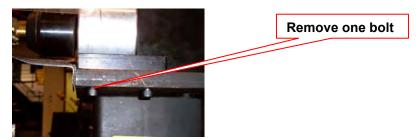
2. Replace the removed bolt with one of the supplied 2" long SHCS as shown below. Tighten the bolt.
