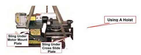
6. Place the machine on your bench, stand or the optional 400-A400 Roller stand. If mounting on your own bench or stand be sure to secure the unit with 3/8" diameter bolts being sure that the bench or stand can support 400 lbs. If you are using the optional roller stand follow the instructions on **page 21** of this manual.
