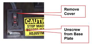
**3.** Remove the Love Joy Cover by removing the two screws. Then loosen the set screws on each half of the Love Joy coupling.
