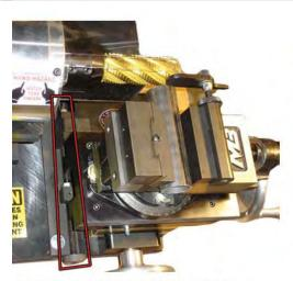
Lower Vise Stop Assembly stops vise table forward movement at preset adjustable vise stop position for proper depth of tube notch.
