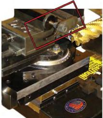
Upper Tube Depth Assembly allows adjustable paddle on magnetic mount to preset tube depth in vise & rotate for cutter clearance.
