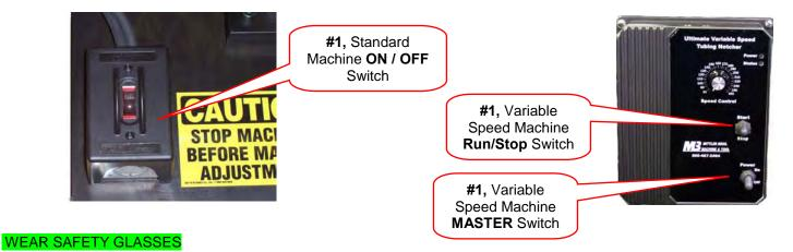
**1.** Be sure your machine is turned off and is plugged into the proper power source. [Both the *Single Speed & Variable Speed* machine operate on 110 Volt single (1) phase electric. Switch is on the left side of the main base plate for single speed and on the control box as shown above.
