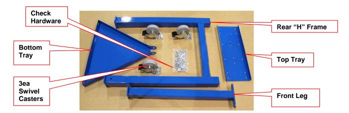
2. Lay the "H" Frame down like shown below. Attach the casters using the 5/16" x 1" bolts, lock washers & nuts. Bolt the remaining caster to the bottom of the front leg as shown. Be sure bolt are installed from the caster side.
