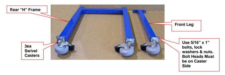
**3.** Attach the bottom tray to the rear H frame using the 3/8" x 3" bolts, lock washers & nuts. Attach the top tray to "H" frame using the 5/16" x 3" bolts, lock washers & nuts.
