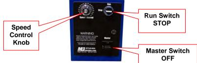
**19.** Turn the **MASTER** switch on and then turn the **RUN** switch on. Turn the speed control knob up and down to cycle the motor. Listen for and clicking or odd sounds. If you here a clicking sound you will need to loosen the spindle housing bolts and then retighten while the motor is running. This will usually align the Love Joy and quiet the clicking.
