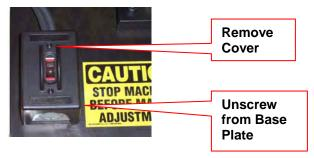
**3.** Remove the Love Joy Cover by removing the two screws. Then loosen the set screws on each half of the Love Joy coupling.
